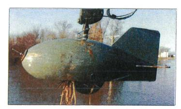
Figure 12: Bed-material samplers are used to collect soil and sediment from river bottoms, a task recommended for a future phase of study
