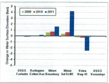
Figure 5: Hydraulic modeling of the 2009, 2010, and 2011 flood events was performed with and without the PER Project elements in place. The Project will minimally impact water surface elevations upstream of Burlington and downstream of Velva, while water surface increases in the developed areas will be contained between the proposed Project leves.
