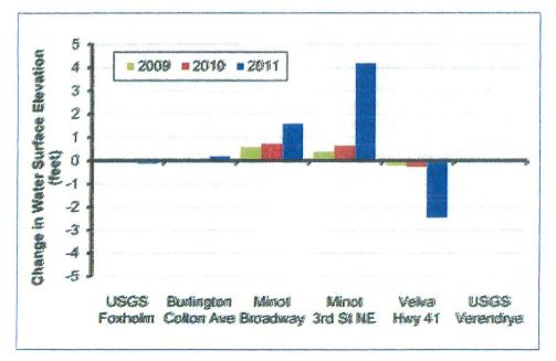
Figure 4: The Project would impress water surface elevations in the vicinity of Minot, but would have minimal impact upstream of Burlington and downstream of Welva.
