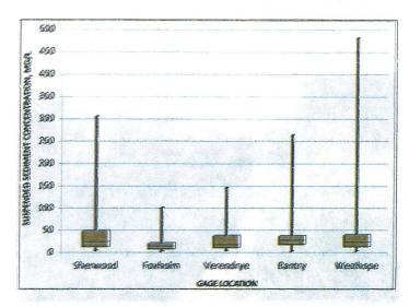
Figure 9: Suspended sediment concentrations vary along the Mouse River but are generally less than 50 milligrams per liter, inclicating that typical flows in the river do not carry large amounts of sediment
