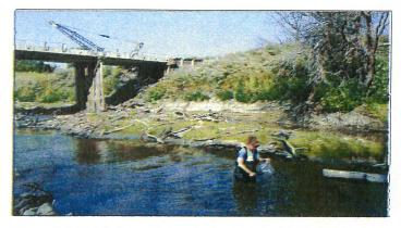
Figure 13: Field channel cross-section surveys include identifying indicators of predominant channel-shaping flows
