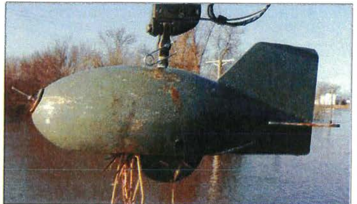
Figure 12: Bed-material samplers are used to collect soil and sediment from river bottoms, a task recommended for a future phase of study
