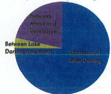
Figure 4: A summary of the primary contributing drainage area and type of flood for the top 28 floods at Verendrye
