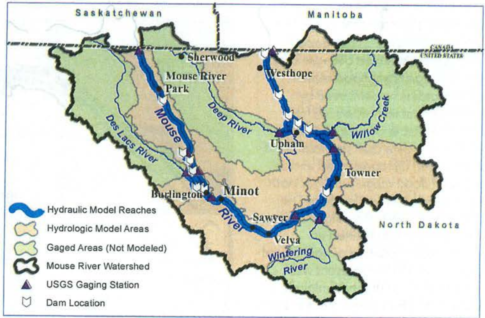
Figure 2: The hydrologic model calculated runoff from ungaged areas of the Mouse River watershed, and the hydraulic model simulated flow in the Mouse River and portions of its four major tributaries.
