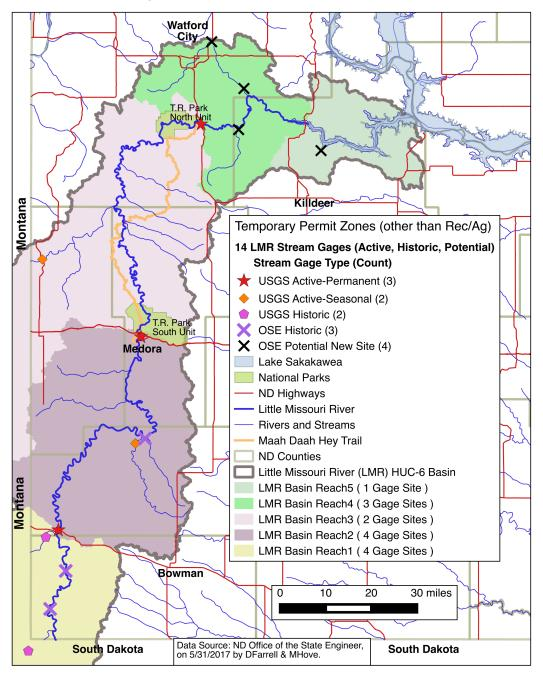
Stream Gage Stations of the U.S. Geological Survey (USGS) and N.D. Office of the State Engineer (OSE) in the Little Missouri River (LMR) Basin.
