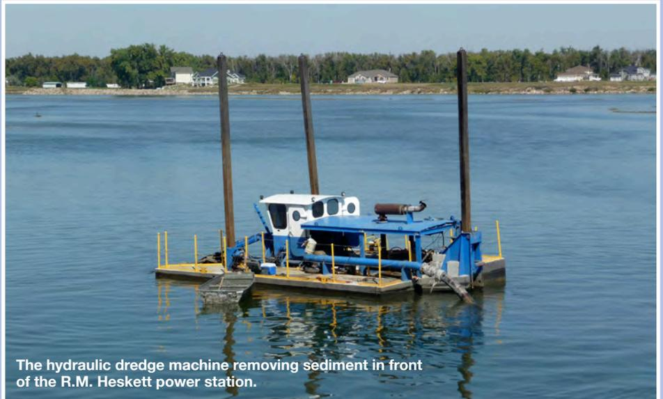
The hydraulic dredge machine removing sediment in front of the R.M. Heskett power station.
