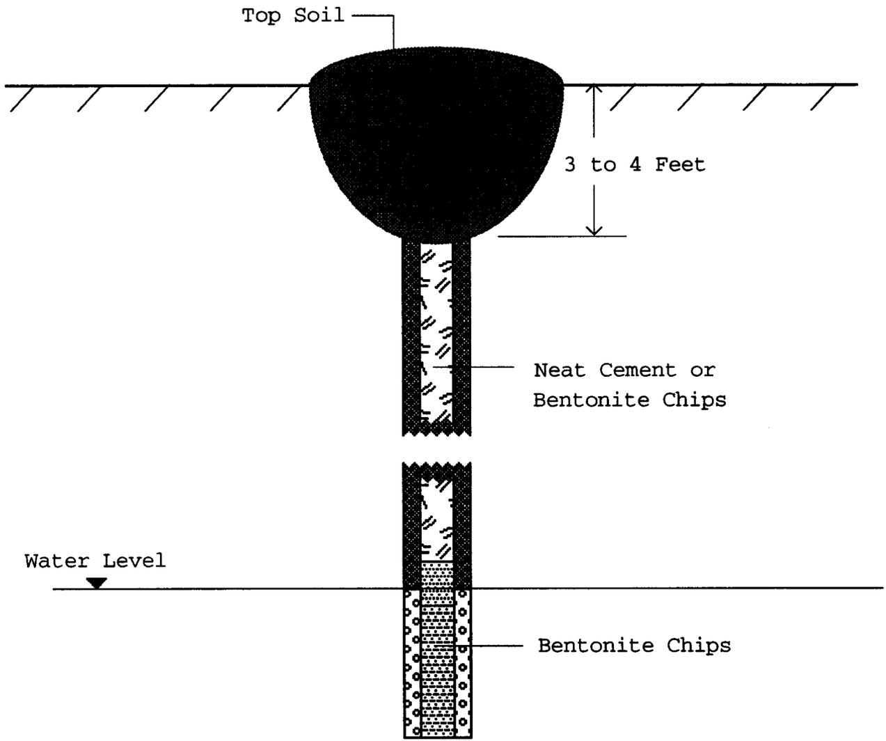
Figure 3. Monitoring well abandonment procedures.
